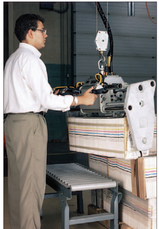
Dual cylinder with side control
