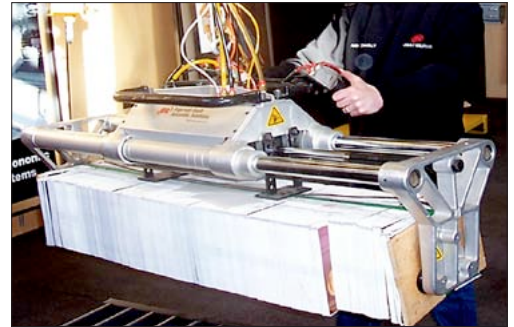
Single cylinder with top swivel handle control
