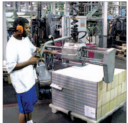
Dual cylinder with top swivel handle control
