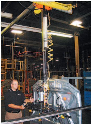
Torque tube with integrated vacuum handling device
